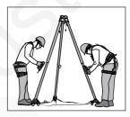
Now install & fix the Universal Brackets on the Tripod Leas to install winch & self- retracting lifeline. further.
