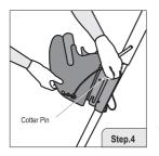
Use solid pin for locking the Retrieval Mounting bracket on pre-installed mounting bracket of tripod leg. Lock the solid pin on mounting brackets using cotter pin.
