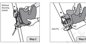
Place the retrieval mounting bracket on the lower mounting bracket pre-installed on the tripod leg and insert the guiding pin into the slot.
